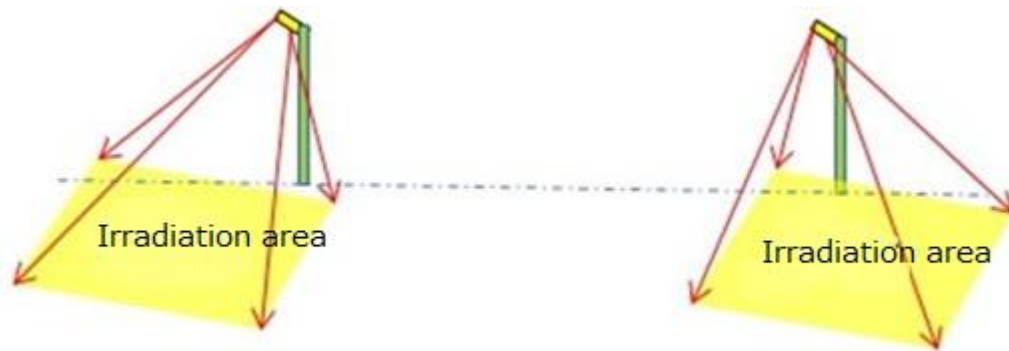
Fig. 5 Illumination distribution with three-dimensional LED lens orientation.
